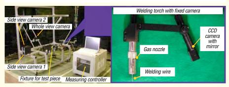
Skill Digitiser<sup>TM</sup> setup for semi-automatic MAG welding
